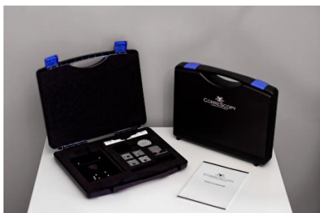
Figure 1. Correscopy setup which comprises multiple sample holders and adapters for various imaging devices supported by the software.
