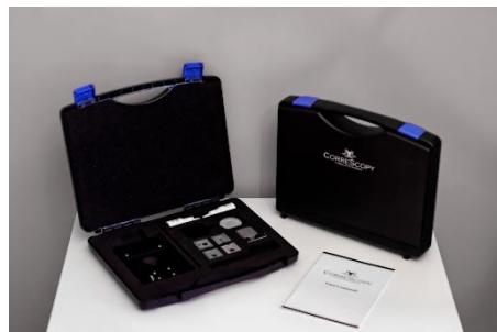
Figure 1. Correscopy setup which comprises sample holders and adapters for various imaging devices supported by the software.
